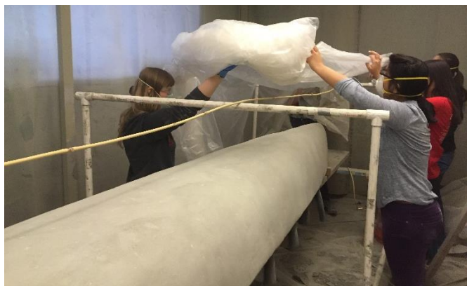
Figure 10. Plastic tent set up. Note the sprinkler hose running along the top of the tent.
