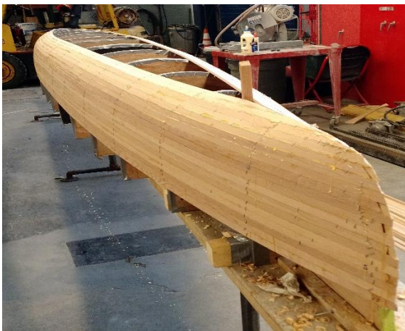
Figure 8. Male mold under construction. The Mold team removed a total of 532 staples upon completion.
