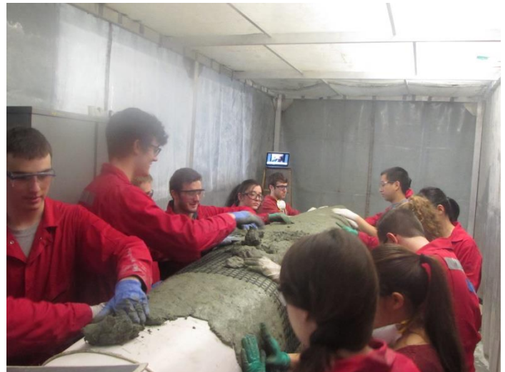
Figure 9. Placement of the Concrete after Mesh Section. Members at the far end of the canoe continue slump boarding and misting the air. Note the ¼ -in rope on the bottom left of the image.
