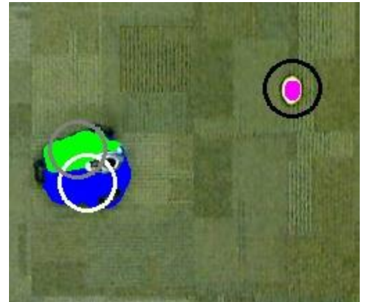
Figure 1: example of our blob detection algorithm detecting the different colored pieces of felt and the lemon.
