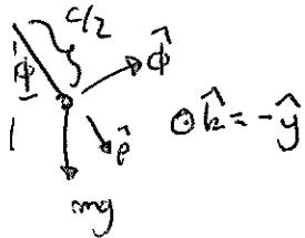
$$\text{usando que } \vec{\tau} = I^g \ddot{\vec{r}} \quad \text{con } \ddot{r}_2 = \dot{\phi} \hat{k} = -\dot{\phi} \hat{y}$$
