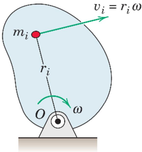
$$T = \frac{M}{2} v_G^2 + \frac{I_G}{2} \omega^2 = \frac{1}{2} (Mr_G^2 + I_G) \omega^2$$
