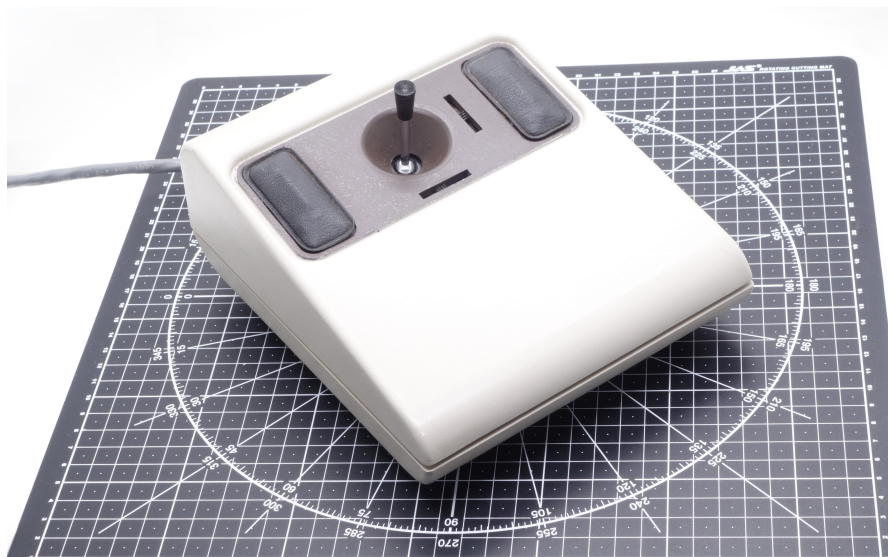
Figure 3: DEC H3060 joystick on a graduated pad with a grid step of 1 cm
