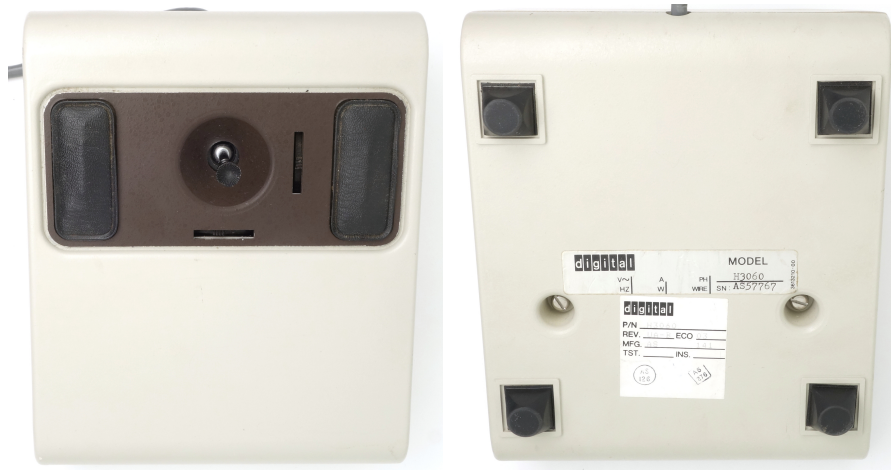
Figure 2: DEC H3060 joystick, top and bottom views
