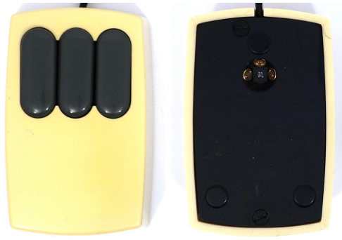
Figure 2: Xerox Alto Optical Mouse, top and bottom views
