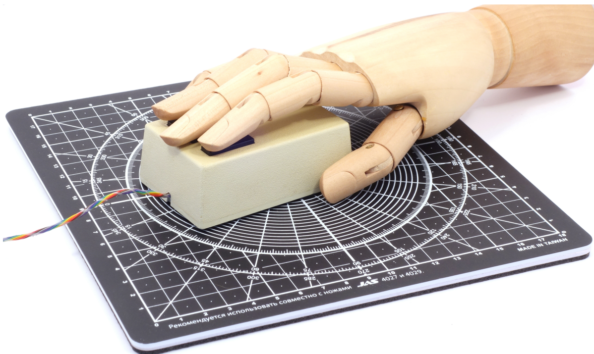
Figure 4: Hawley Mark II with a human hand model
