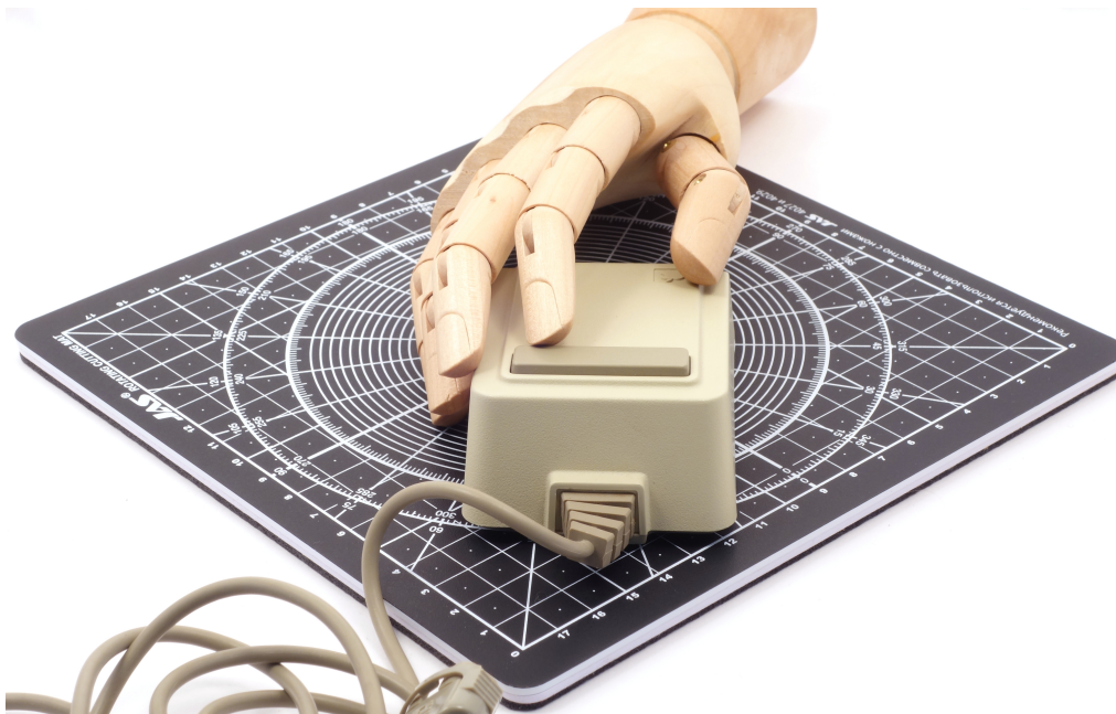
Figure 4: Apple Lisa mouse with a human hand model
