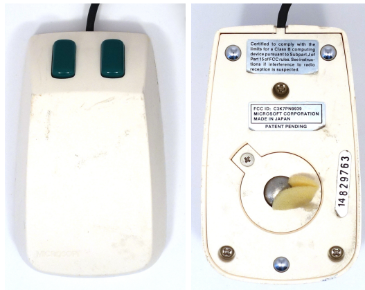
Figure 2: Microsoft Green Eyed Mouse, top and bottom views
