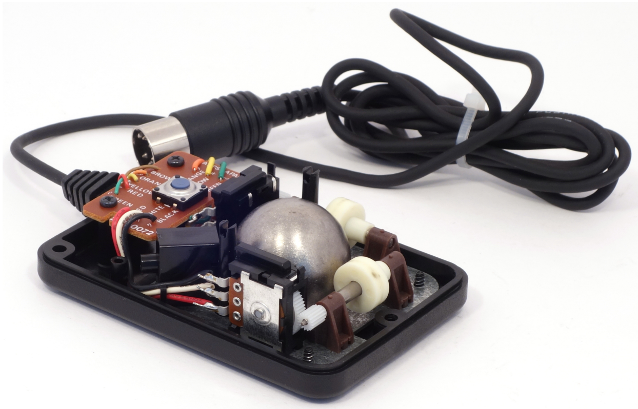
Figure 5: Tandy Color Mouse disassembled
