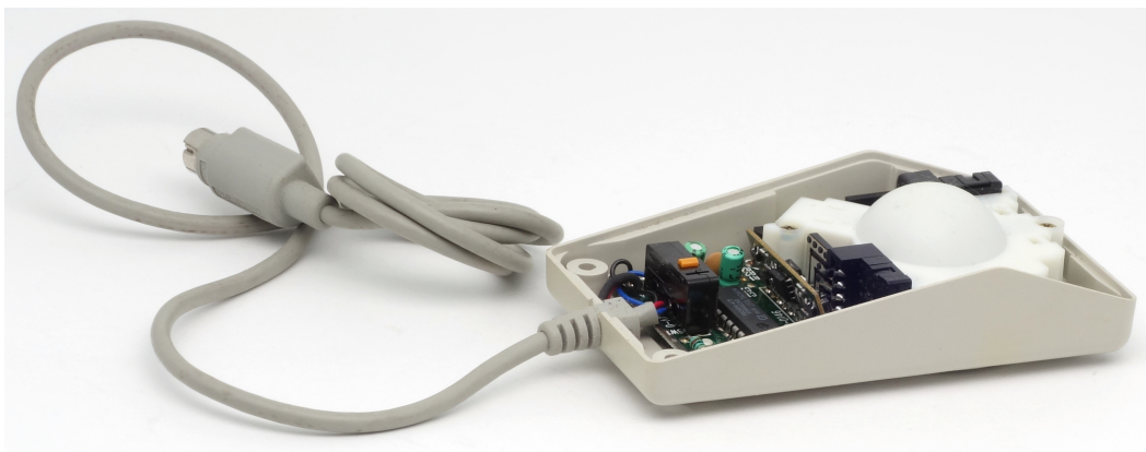
Figure 5: Apple Desktop Bus Mouse disassembled
