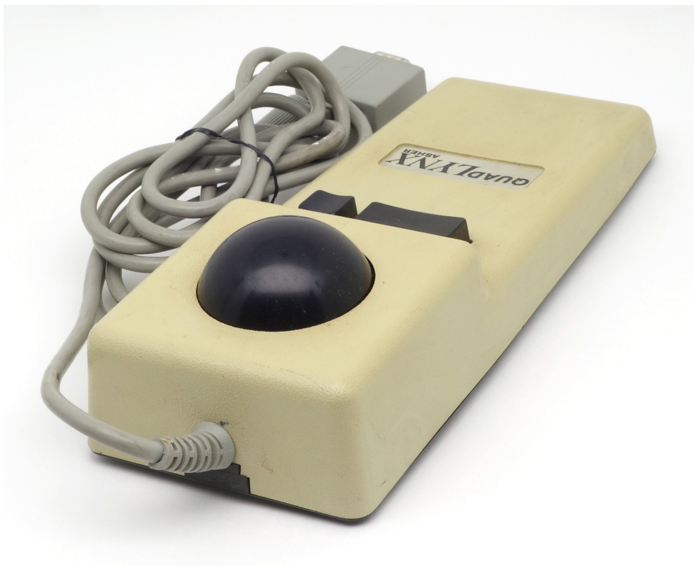
Figure 1: Asher quadLYNX trackball
