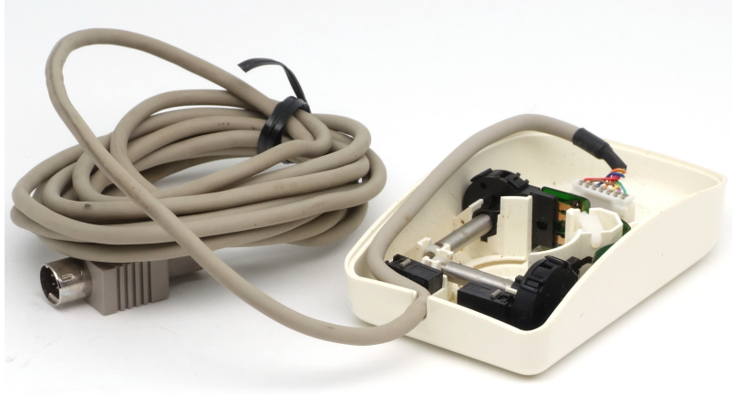
Figure 5: Microsoft Dove Bar Mouse disassembled
