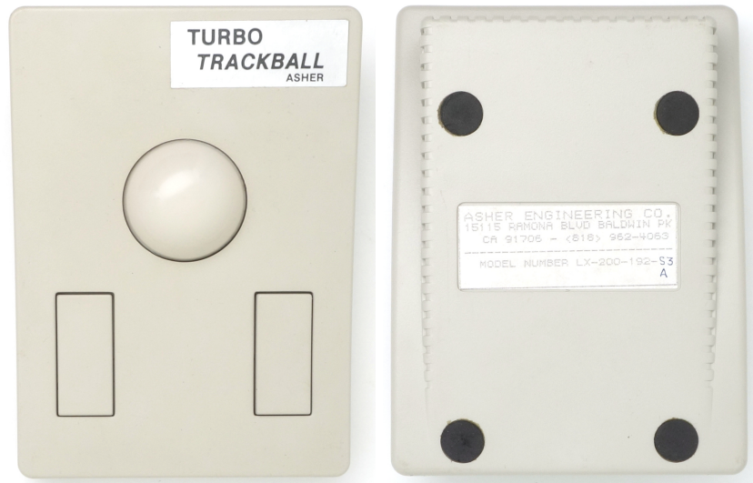
Figure 2: Asher Turbo trackball, top and bottom views
