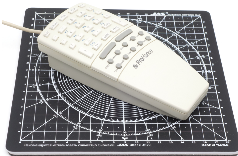
Figure 4: Prohance PowerMouse 100 on a graduated pad with a grid step of 1 cm
