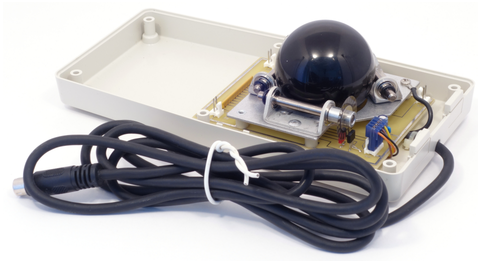
Figure 5: Diamond XL trackball disassembled
