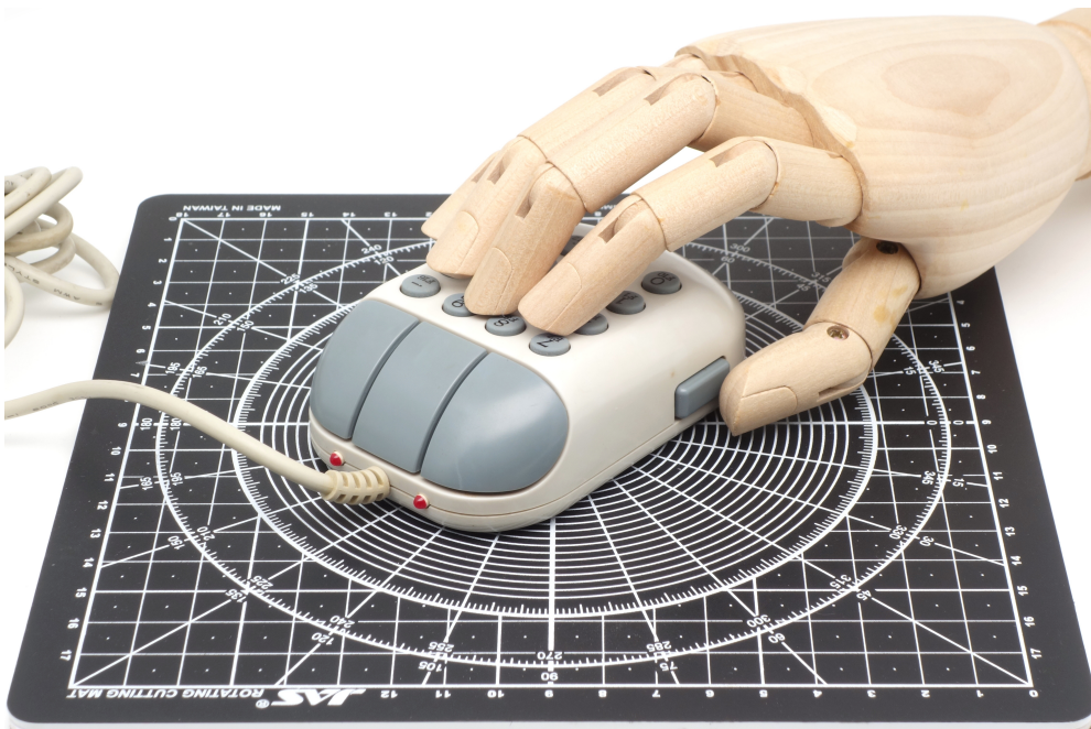
Figure 5: Mariqua Mouse with a human hand model, pressing the keys
