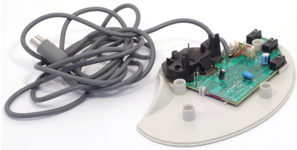
Figure 5: Logitech TrackMan trackball disassembled
