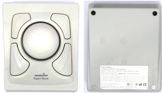
Figure 2: Kensington Expert Mouse Trackball, top and bottom views
