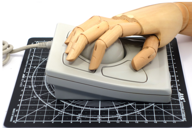
Figure 4: Kensington Expert Mouse Trackball with a human hand model
