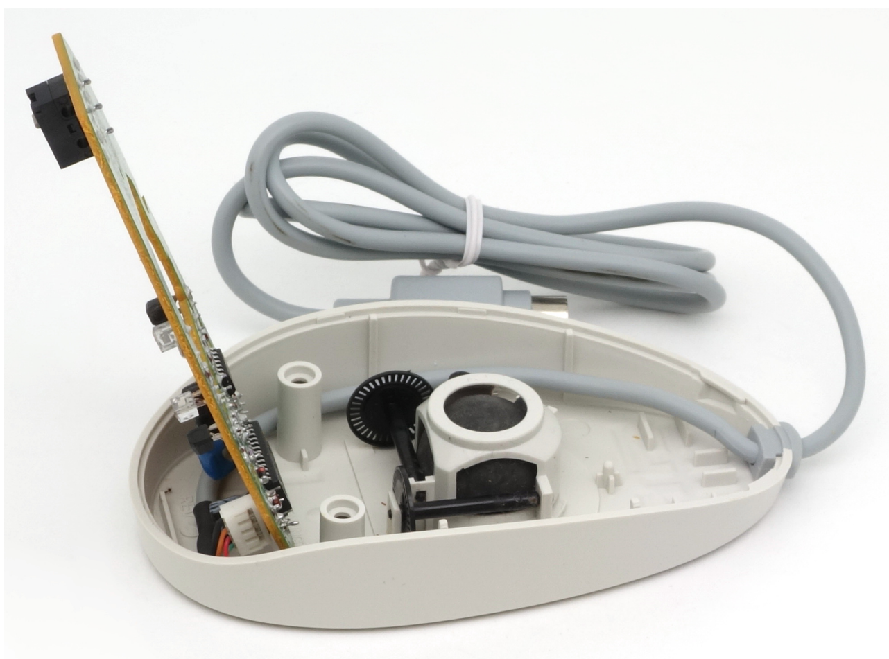
Figure 5: Kensington Mouse 2nd generation disassembled
