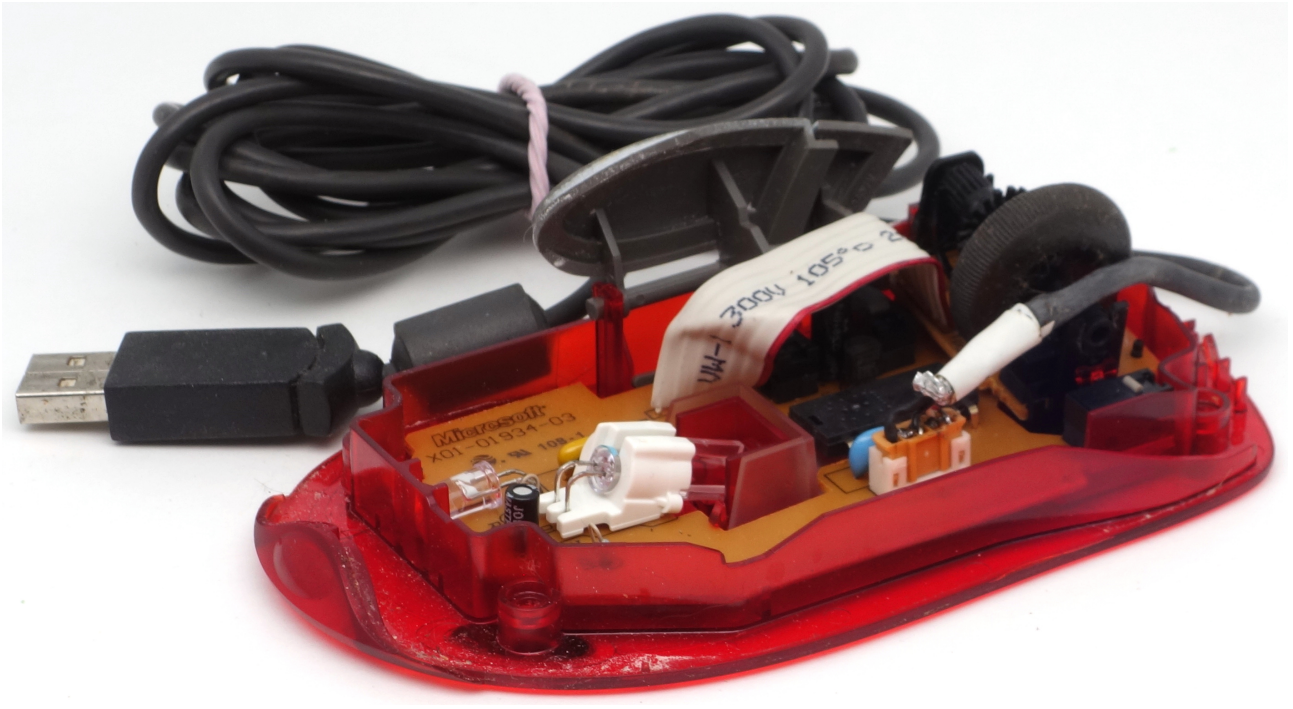
Figure 5: Microsoft IntelliMouse Explorer mouse disassembled
