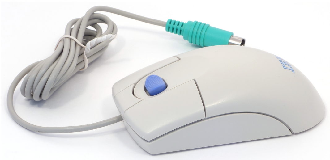
Figure 1: IBM ScrollPoint II mouse
