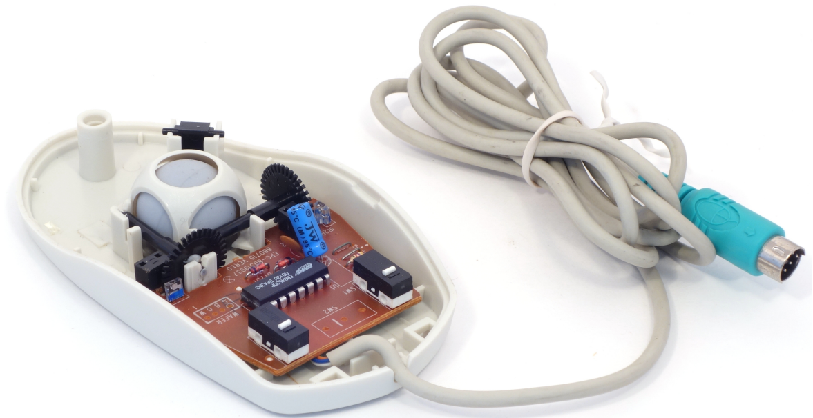
Figure 5: SurfMouse mouse disassembled
