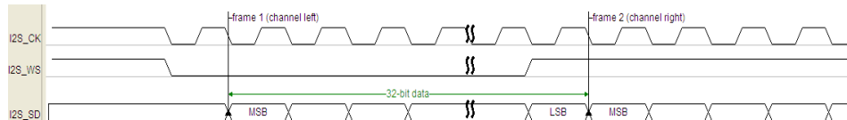
Figure 15-10. I2S Phillips standard timing diagram (DTLEN=10, CHLEN=1, CKPL=1)
