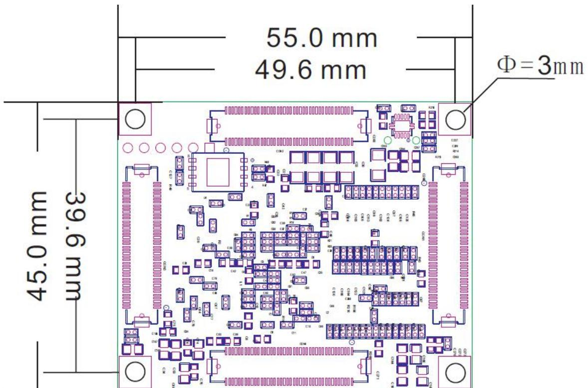
Figure 12-2: AC7100B FPGA Core board (Bottom view)
