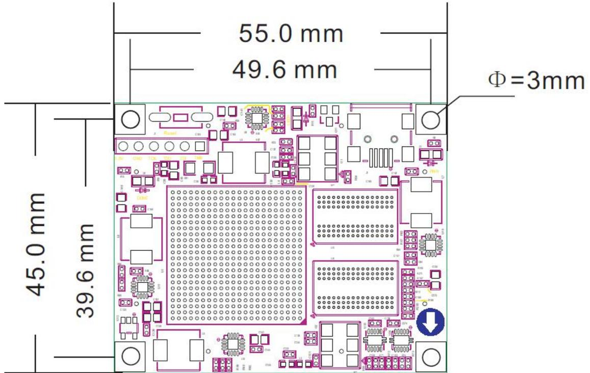
Figure 12-1: AC7100B FPGA Core board (Top view)
