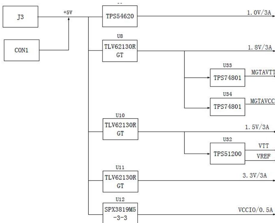
Figure 11-1: Power Supply on core board schematic
