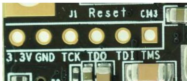
Figure 8-2 JTAG Interface on Core Board
