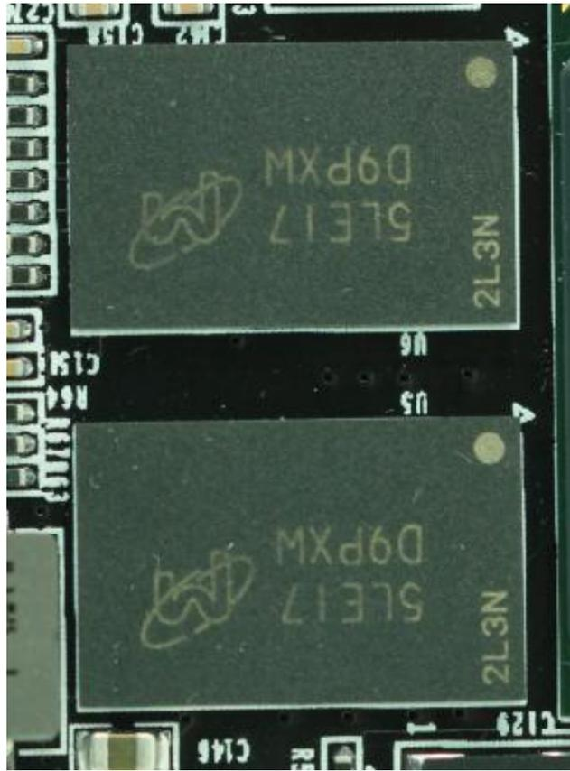
Figure 4-2: The DDR3 on the Core Board
