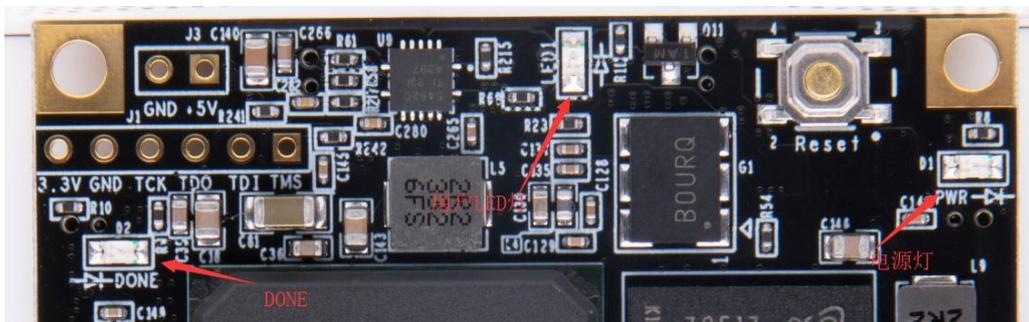
Figure 6-2: LED lights on the Core Board
