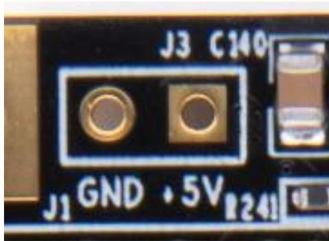
Figure 9-1: Power Interface on the Core Board
