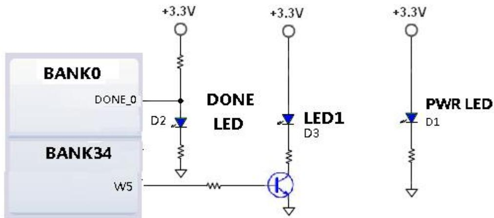
Figure 6-1: LED lights on core board Schematic
