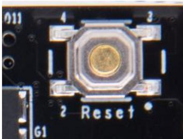
Figure 7-2: Reset button on the Core Board
