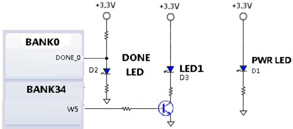
Figure 6-1: LED lights on the Core Board Schematic
