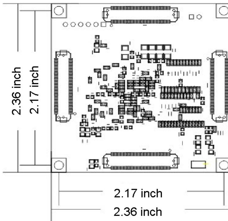
Figure 11-2: AC7A035 FPGA Core board (Bottom View)
