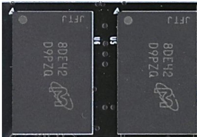
Figure 4-2: The DDR3 on the Core Board
