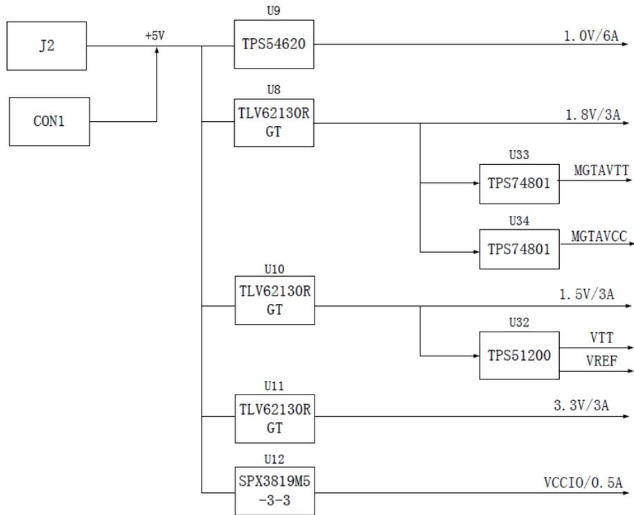
Figure 10-1: Power Supply on core board schematic
