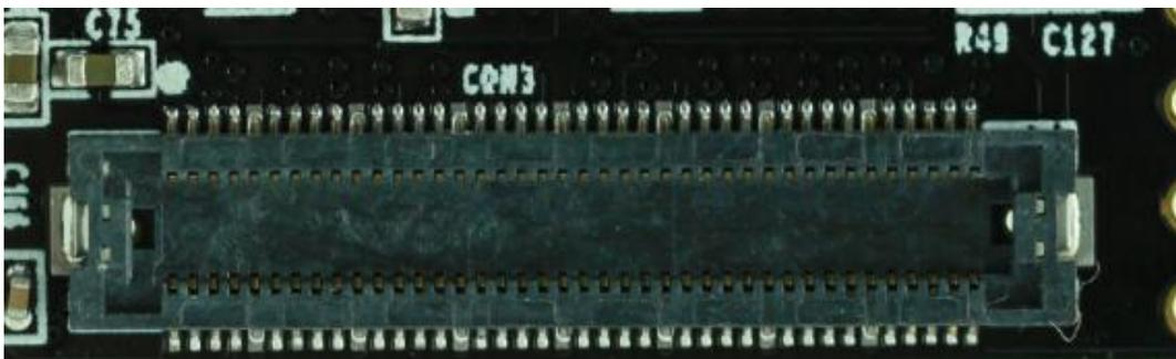
Figure 9-3: Board to Board Connectors CON3 on the Core Board
