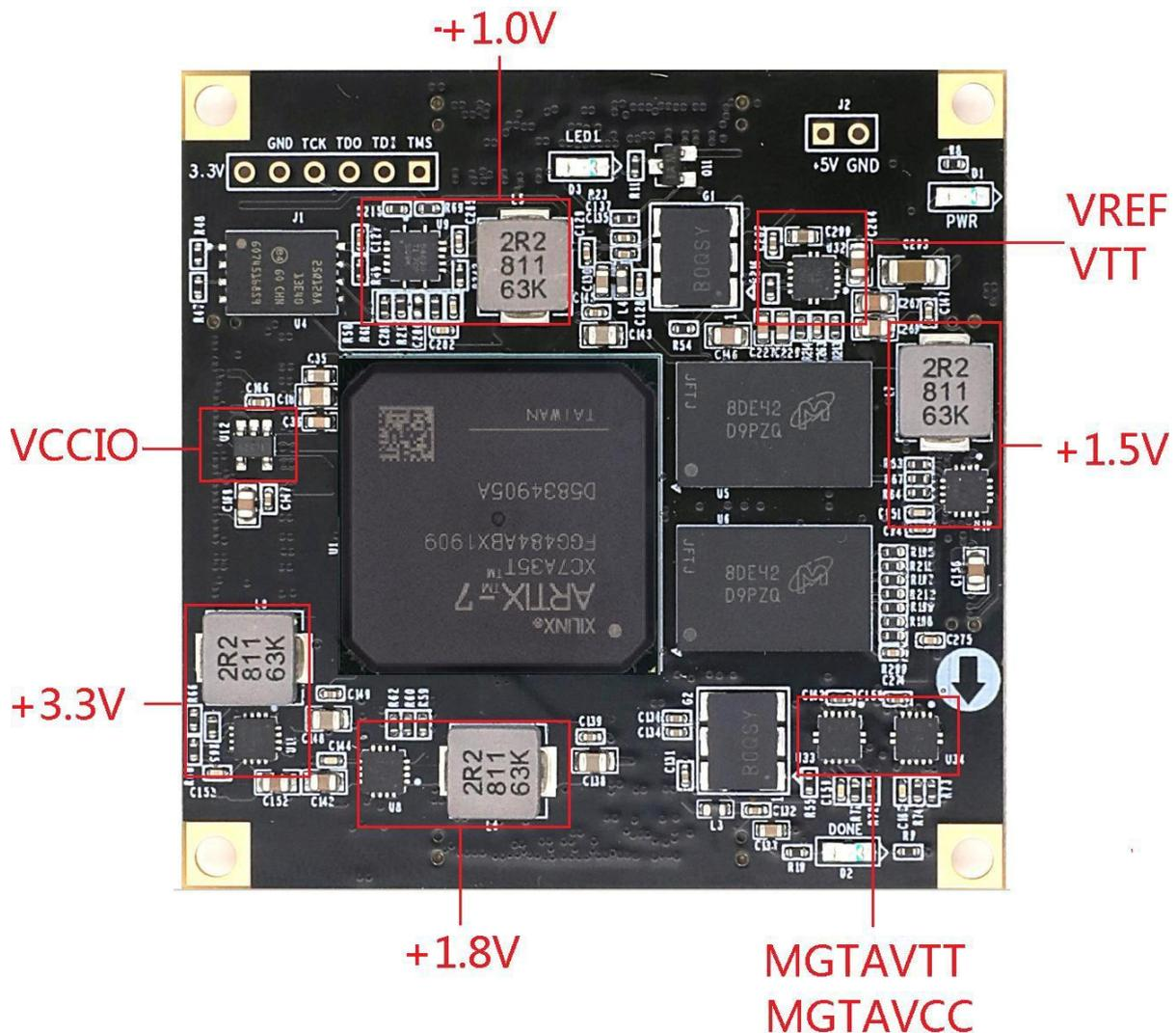
Figure 10-2: Power Supply on the AC7A035 FPGA Core Board
