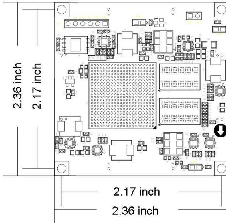
Figure 11-1: AC7A035 FPGA Core board (Top View)
