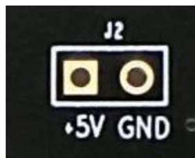
Figure 8-2: Power interface on the Core Board
