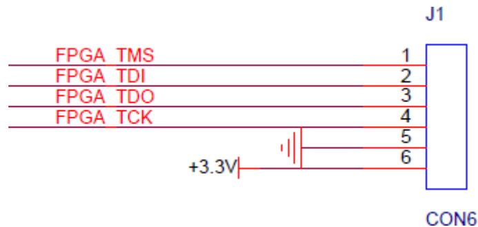
Figure 7-1: JTAG Interface Schematic
