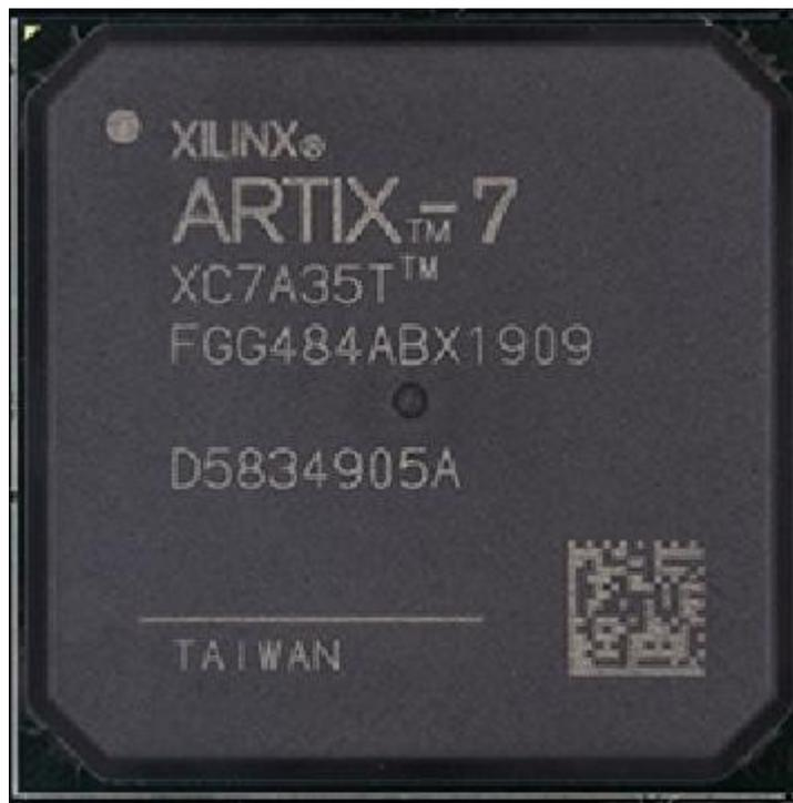
Figure 2-2: FPGA chip on board
