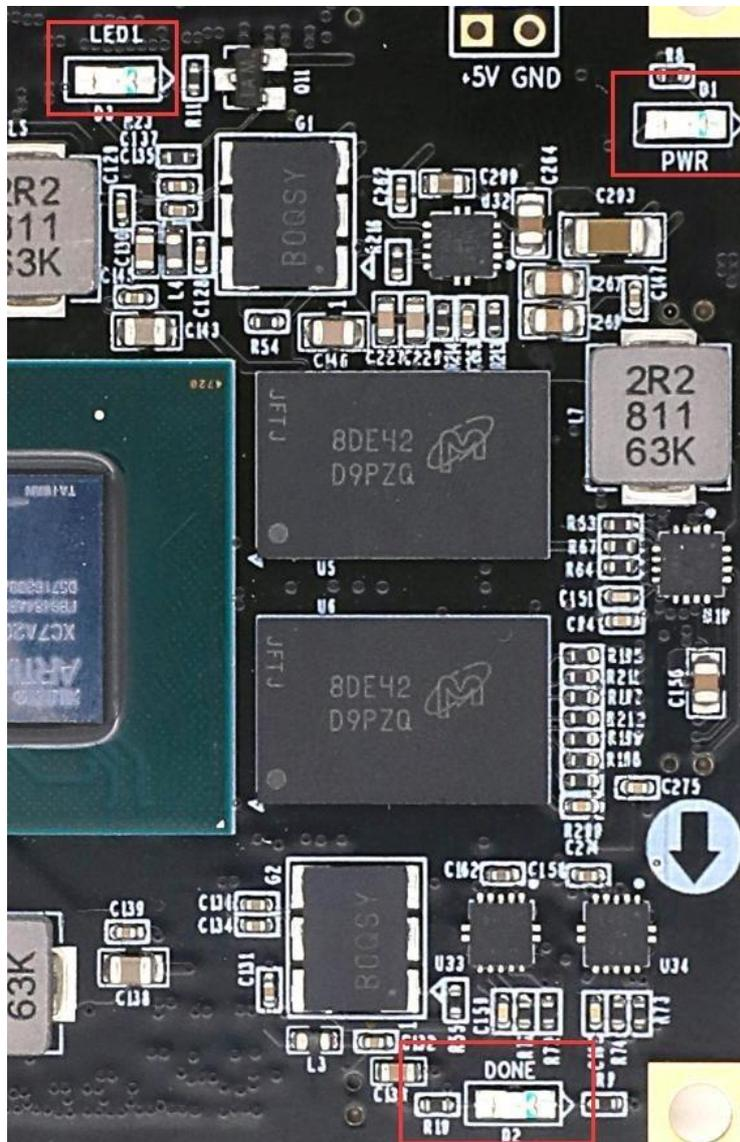
Figure 6-2: LED lights on the Core Board
