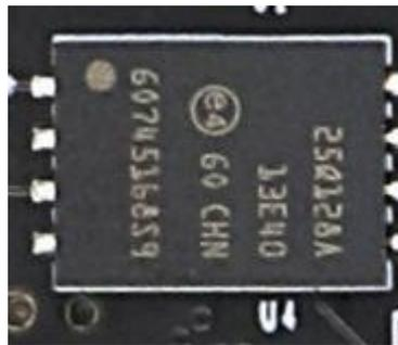
Figure 5-2: QSPI FLASH on the Core Board
