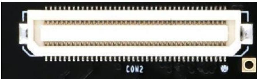
Figure 9-2: Board to Board Connectors CON2 on the Core Board
