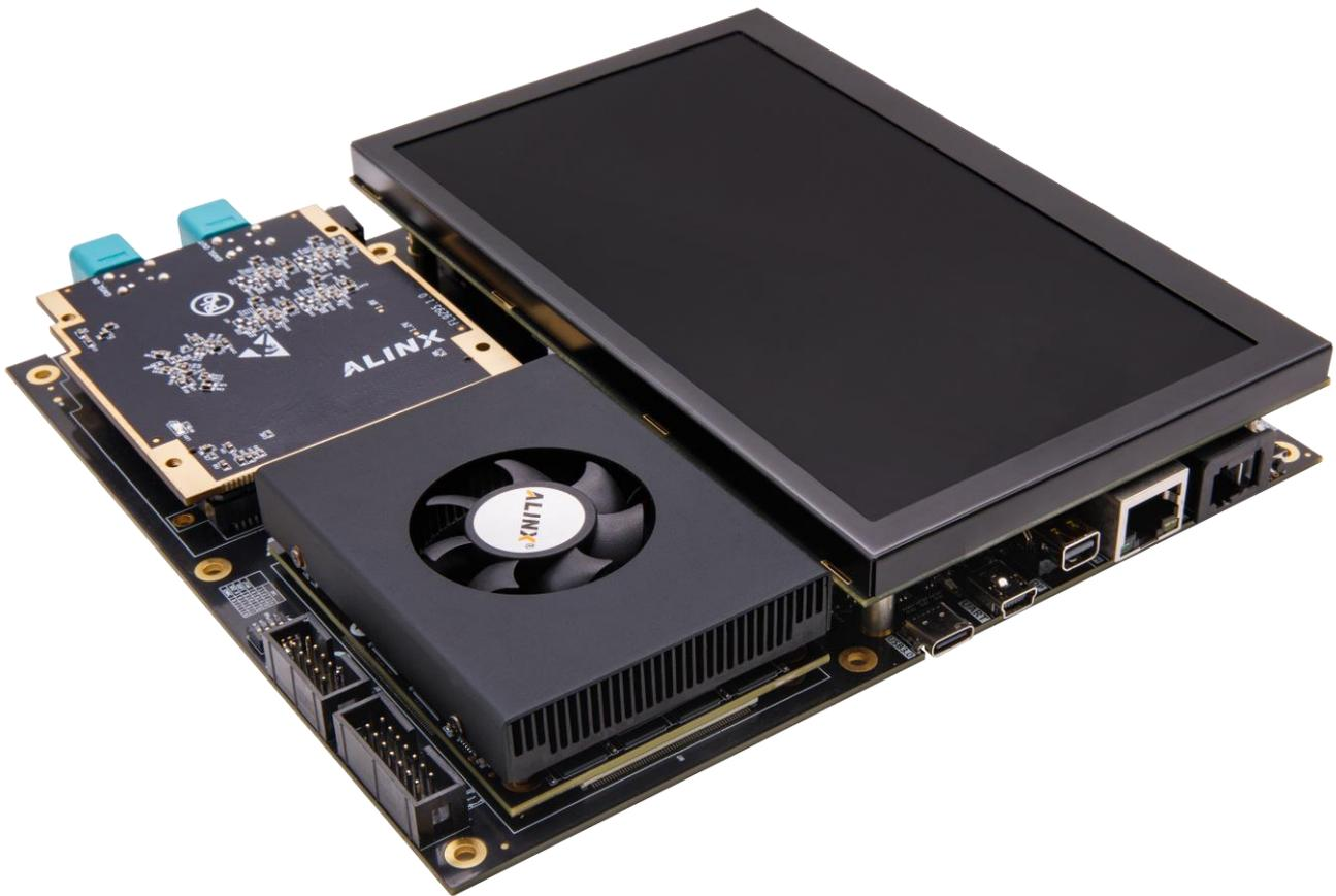
Figure 2.2 Connection between the Z7-A development board and the LCD screen
