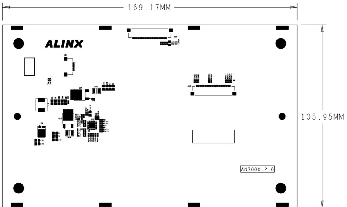
**Figure 1- Module dimensions**
