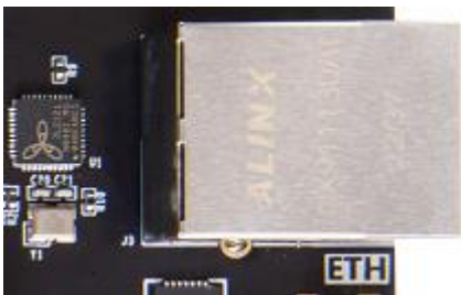
Figure 16: Physical Diagram of Ethernet PHY Chip
