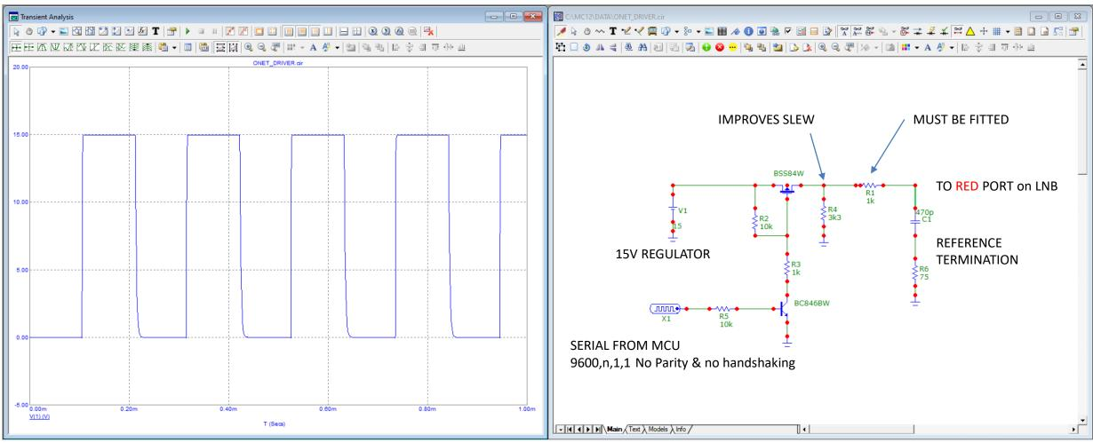
15V +/-1V voltage source is needed and this can be a linear regulator or even a simple Zener Diode regulator. Its recommended to use a FET as the series switch and to fit a load (R4) to improve the slew rate on the falling edges. R1 is the required 1k resistor and C1/R6 provide a termination to the internal reference to reduce any pulling and pushing of the reference. Keep C1 below 1nF so it doesn't degrade the slew of the data.
