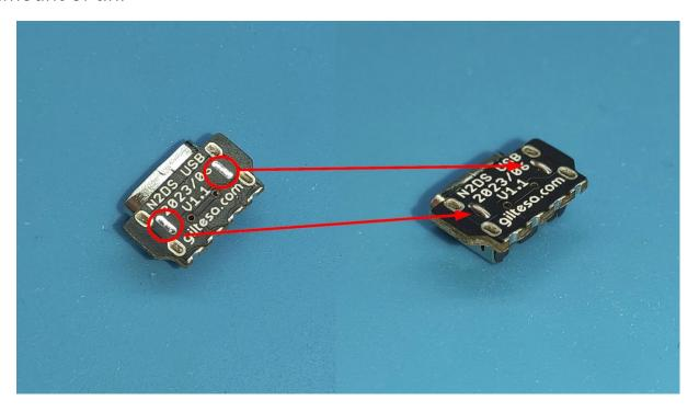
These pads will align with the large holes on the original connector. It is crucial that these two pads are soldered securely as they serve as the main points of support for the board.
