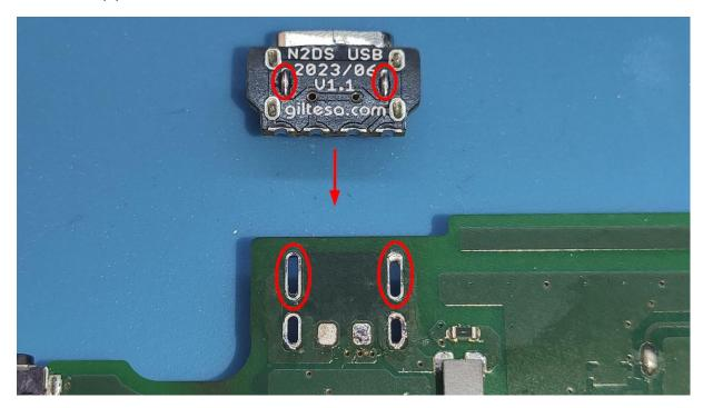
Align the board properly and solder the first pad on the bottom side. Then, double-check that the boards are still well aligned and solder the other one.
