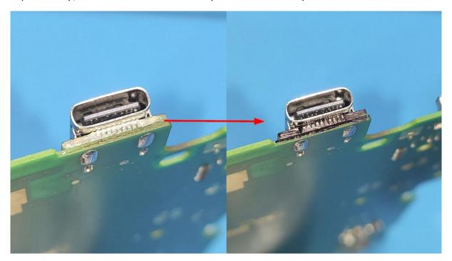
Before reassembling everything, you can connect the USB-C cable to the connector and observe if the orange light turns on for a few seconds and then turns off. This confirms that the installation is perfect.
