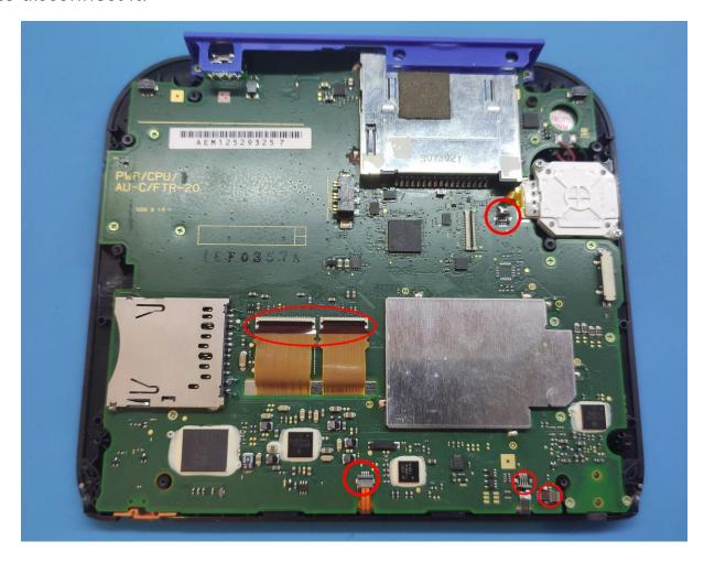
Then, remove the last fourteen screws (Be careful with the two lower screws, they are shorter than the rest)
