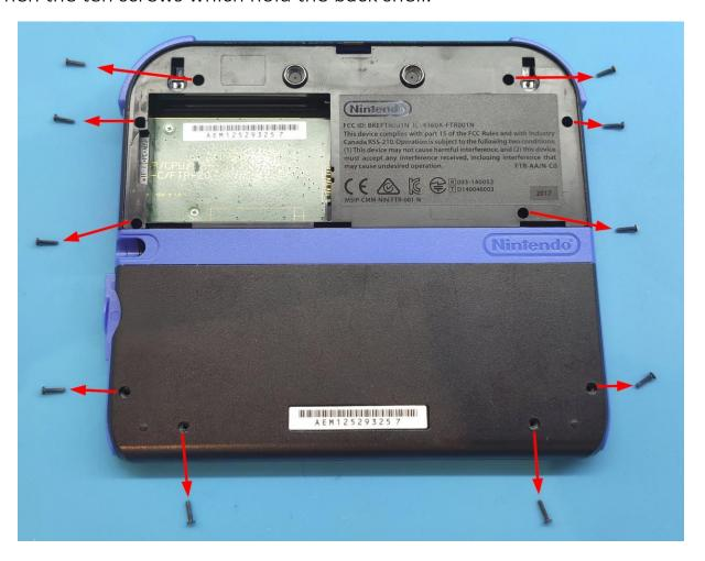
Open the back shell carefully because it is connected to the mainboard with one flex cable. To remove it, lift the plastic retainer and pull back the cable.
