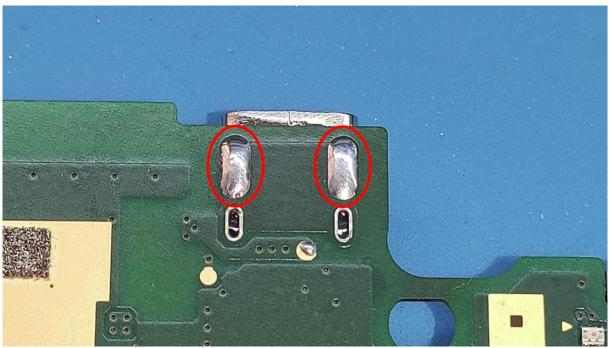
The board should be completely flat against the Nintendo 3DS mainboard, without any gaps in the middle.
