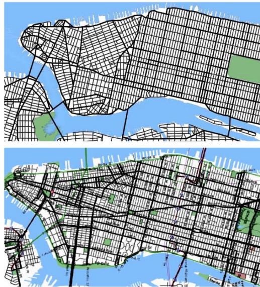
Figure 1: CityEngine is used to generate roads on Manhattan Island, New York, United States (top), versus the real-life road layout (Parish and Müller, 2001).
