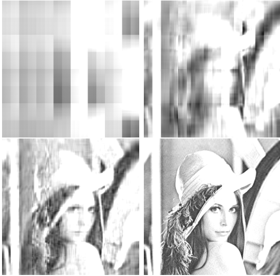
Figure 11: Compressing an image with an MPS. Clockwise from top left: \chi = 2 , \chi = 9 , \chi = 20 , \chi = 100 , with compression ratios of 1927.5, 126.2, 31.3, and 2.24, respectively. Lossless storage as an MPS results in a compression ratio less than 1.
