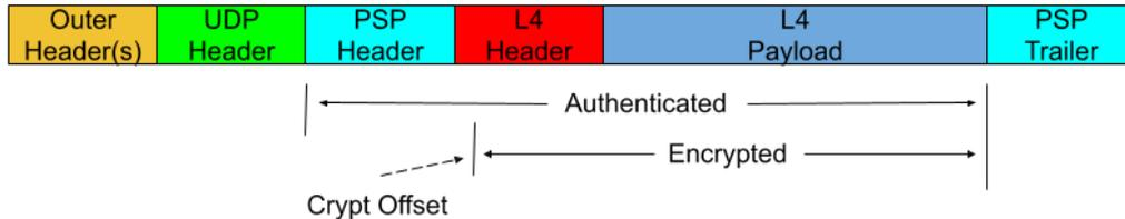
A more specific example of the most common format of a PSP packet in transport mode is shown in the figure below. In the specific example, the outer header is IPv6. Support must also be provided for encapsulations where the outer header is IPv4. Flexibility to support additional outer encapsulation formats is desired (examples include GRE and MPLS).
