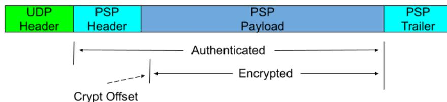
The format of the PSP packet is shown in the figure above. Currently, PSP packets are always encapsulated in a UDP packet, but alternative encapsulations may be used in the future.
