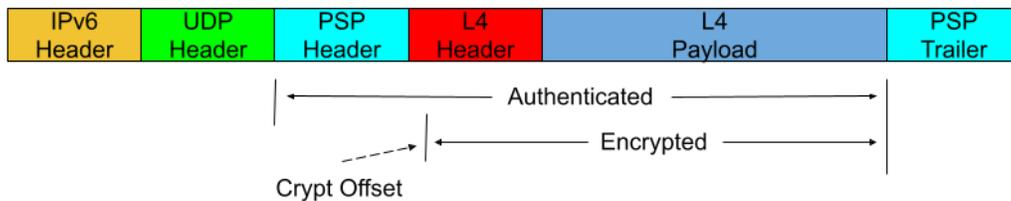
The transport mode packet format is typically used in non-virtualized environments.
