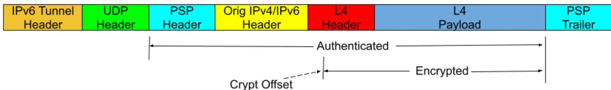
The tunnel mode packet format is typically used in virtualized environments.
