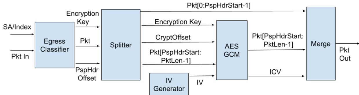
On transmit, PSP packet processing can be implemented as shown by the example block diagram in the figure above. The egress classifier is responsible for outputting the encryption key and building the PSP encapsulation (including the PSP and UDP headers). The encryption key can be produced in multiple ways:
