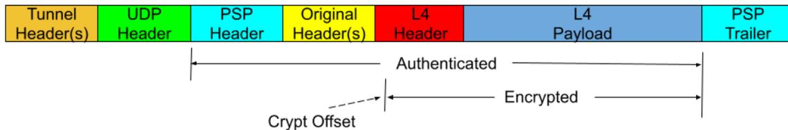
A more specific example of the most common format of a PSP packet in tunnel mode is shown in the figure below. In the specific example, the tunnel header is IPv6, and the original packet is IPv4/IPv6. Flexibility to support additional encapsulation formats is desired.
