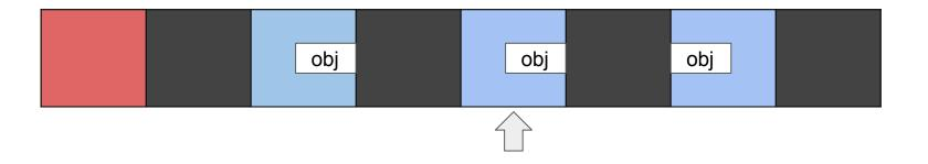
Depending on object placement (left or right), either overflow or underflow accesses will result in page faults. GuardAlloc() may randomly choose left or right placement.
