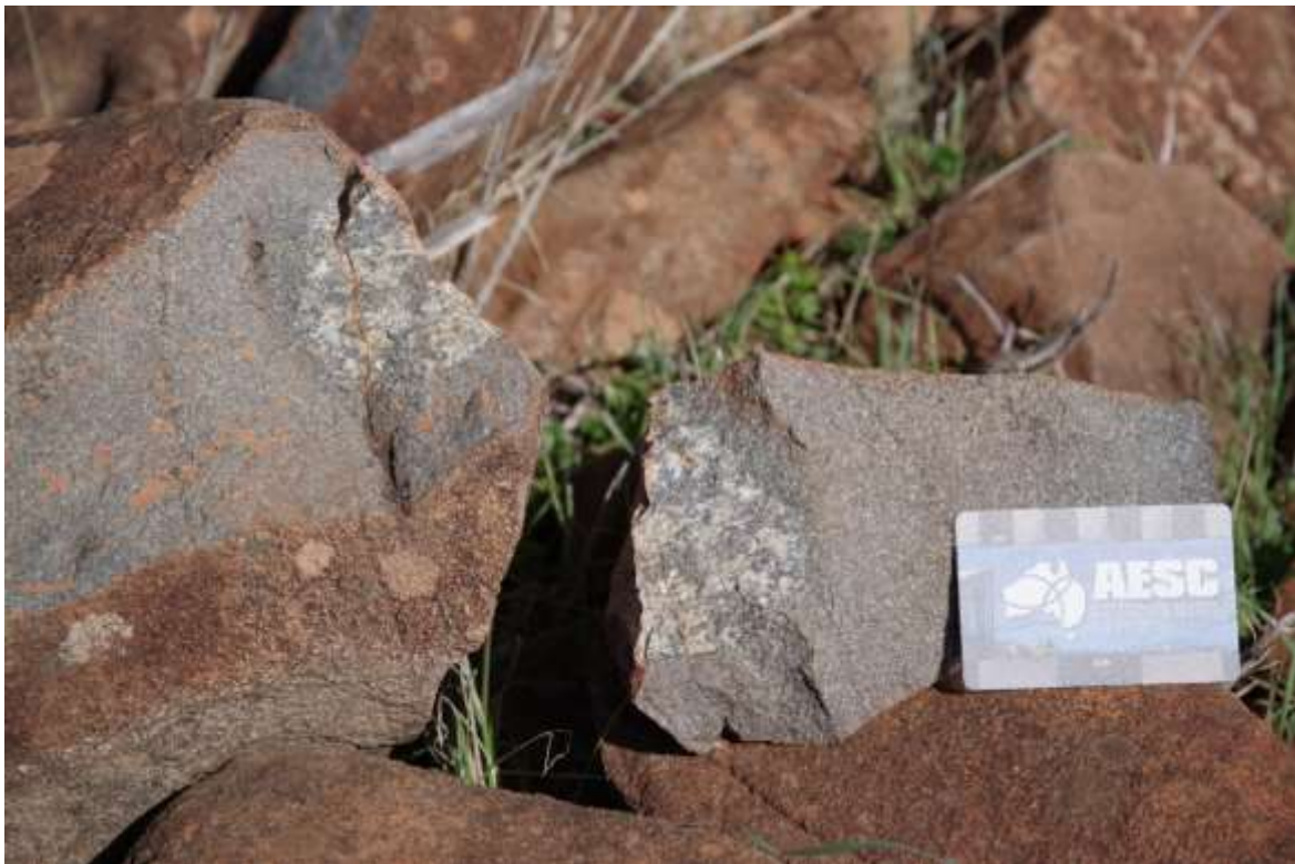
Figure 27. “Quartz diorite”(?) dyke with grey granitic gneiss clasts, mag sus 5 - 10 \times 10^{-5} SI (image 7849, locality GB203)
