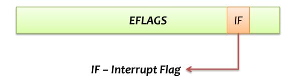
The IF flag inside EFLAGS controls the system interrupts. If set, the system accepts interrupts, else it ignores the interrupt signal.
