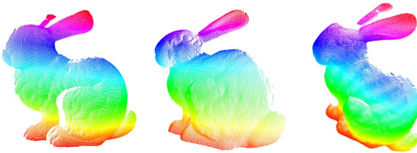
(a) Data point cloud. (b) Model point cloud. (c) Merged View. Figure 16 Bunny model with continuous hue variation in one axis.
