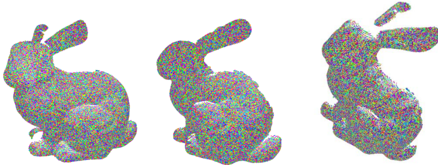
(a) Data point cloud (b) Model point cloud (c) Merged View Figure 18: Bunny point cloud with randomized hue distribution
