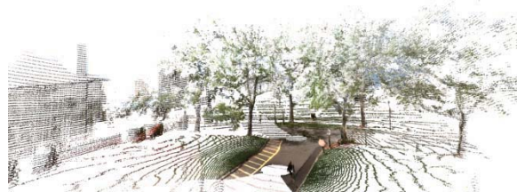
(b) Coordinate data and color data from both the vantage points Figure 11: Color point cloud map generated from two vantage points after registration.
