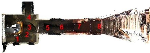
Figure 19. Eight scans aligned to form a complete map a building hallway with approximately five million points.
