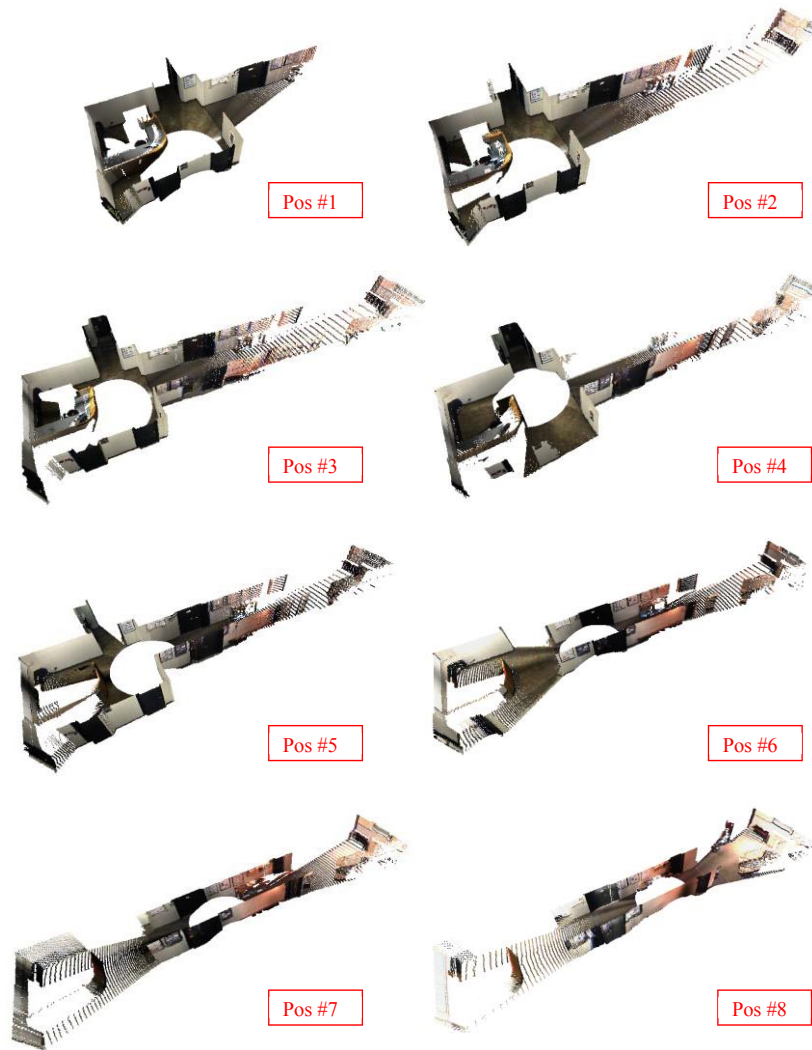
Figure 17. Color point clouds generated at 8 different vantage positions in building hallway.
