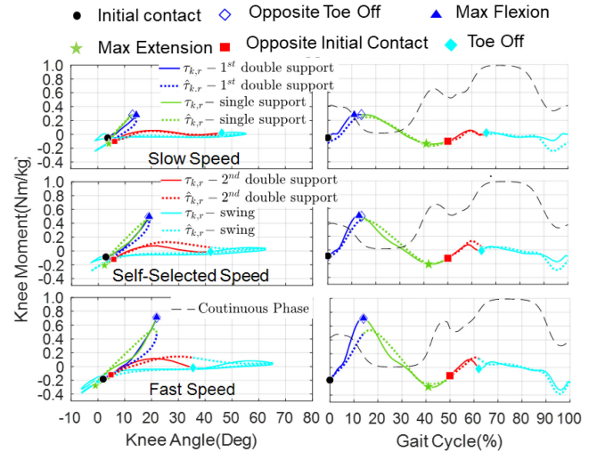
Fig. 9. Demonstration of the continuous-phase stiffness model (see Fig. 7) in one subject. The left column depicts the knee angle versus the estimated knee moment, and the right column depicts the gait cycle versus the estimated knee moment. The blue color indicates the single-support phase, the red color indicates the second double-support phase, and the cyan color indicates the swing phase. The solid line represents the biological knee moment, whereas the dashed line represents the estimated knee moment. The top, middle, and bottom rows show the slow, self-selected, and fast walking speed results, respectively. The black dashed line in the right column depicts the value of the sigmoid function S(\theta_{k,r}, \theta_{k,l}) \in [0, 1] in (11) across the entire gait cycle. It shows that the stiffness model is more inclined to the stance-phase model during the first double-support and single-support phases, whereas the swing-phase stiffness model has a higher weight during the second double-support and swing phases.
