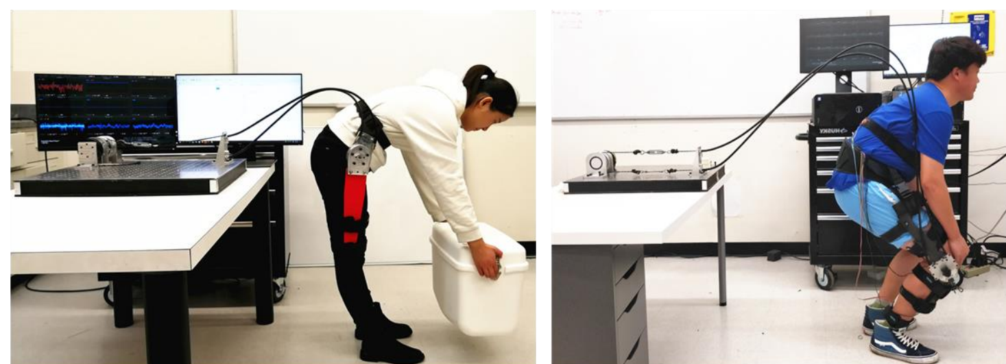
Omni-Hip72 72 Nm peak torque Hip (tethered) Omni-Knee72 72 Nm peak torque Knee (tethered)
