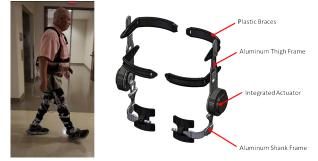
Fig. 2. Mechanical design of our portable knee exoskeleton. The knee exoskeleton was able to provide walking assistance to an elderly subject
