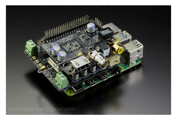
3. Works independently as a S/PDIF FIFO by integrating with a ReceiverPi and a FifoPi (RaspberryPI free )
