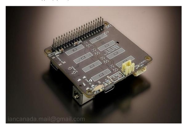
3. ConditionerPi with ultra capacitors installed
