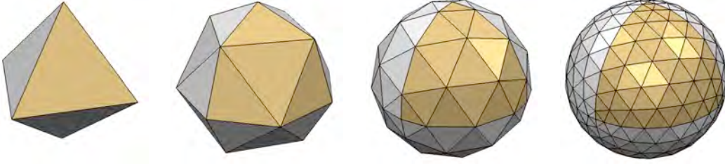
Figure 2.3: Each subdivision step halves the edge lengths, increases the number of faces by a factor of 4, and reduces the error by a factor of \frac{1}{4} .
