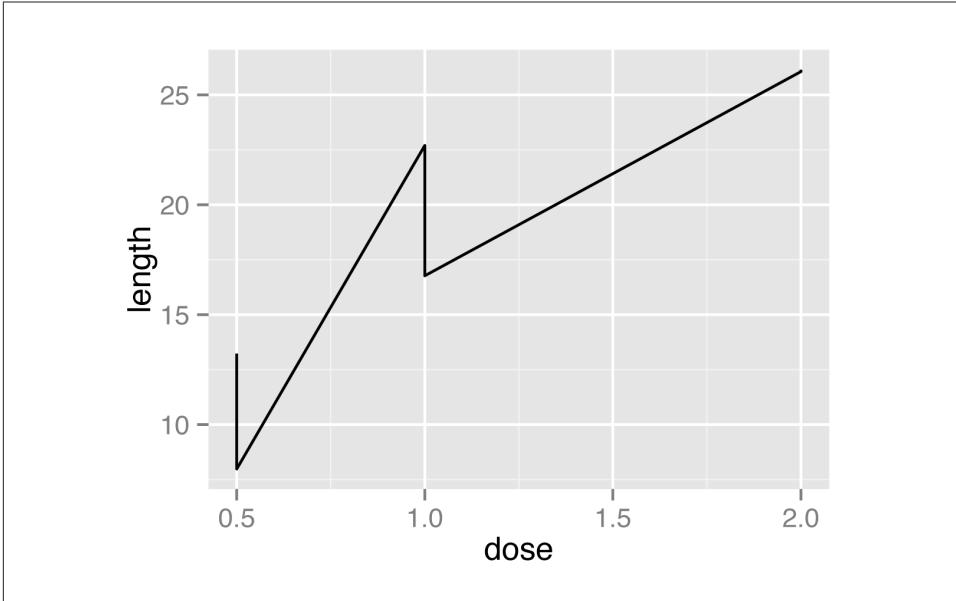
Figure 4-8. A sawtooth pattern indicates improper grouping
