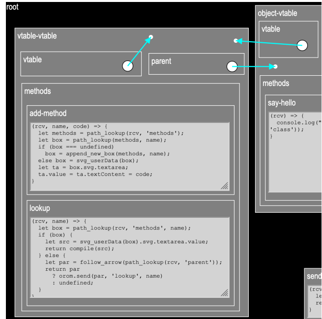
Figure 2: Part of Id/SVG: Obj-dicts are moveable and resizable nested boxes, referencing each other via real arrows.
