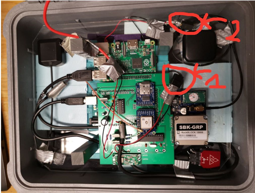
Figure 3: The main power connectors are highlighted in red. Connect them fully and securely, and the instrument will start. Depending on the exact instrument, either the connector shown, or a slightly different connector model, may be used. Feel free to rip off the tape holding the connectors, this is only used to secure everything during transport. The connectors can only be inserted in the right polarisation direction.
