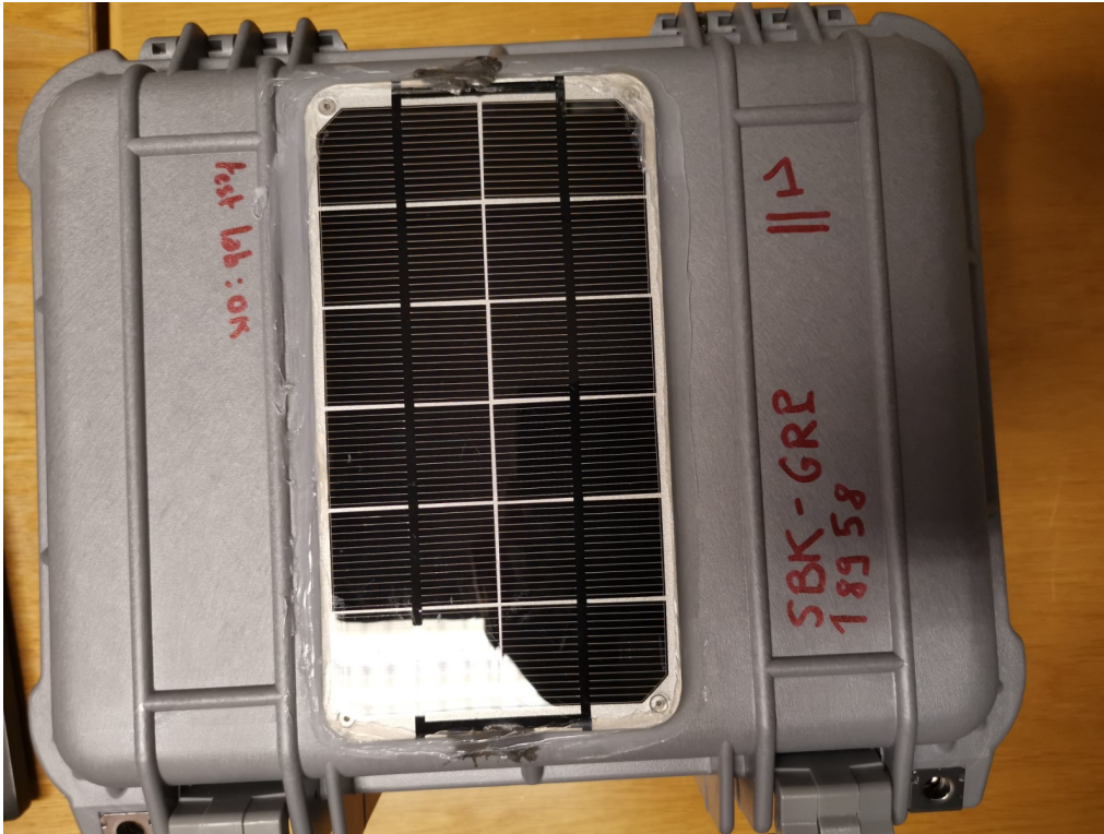
Figure 1: The instrument seen from the top, with solar panel, and a written copy of the Iridium modem reference number (here, SBK-GRP 18958). In addition, each instrument in a production series is given a number, here this is instrument number 1.
