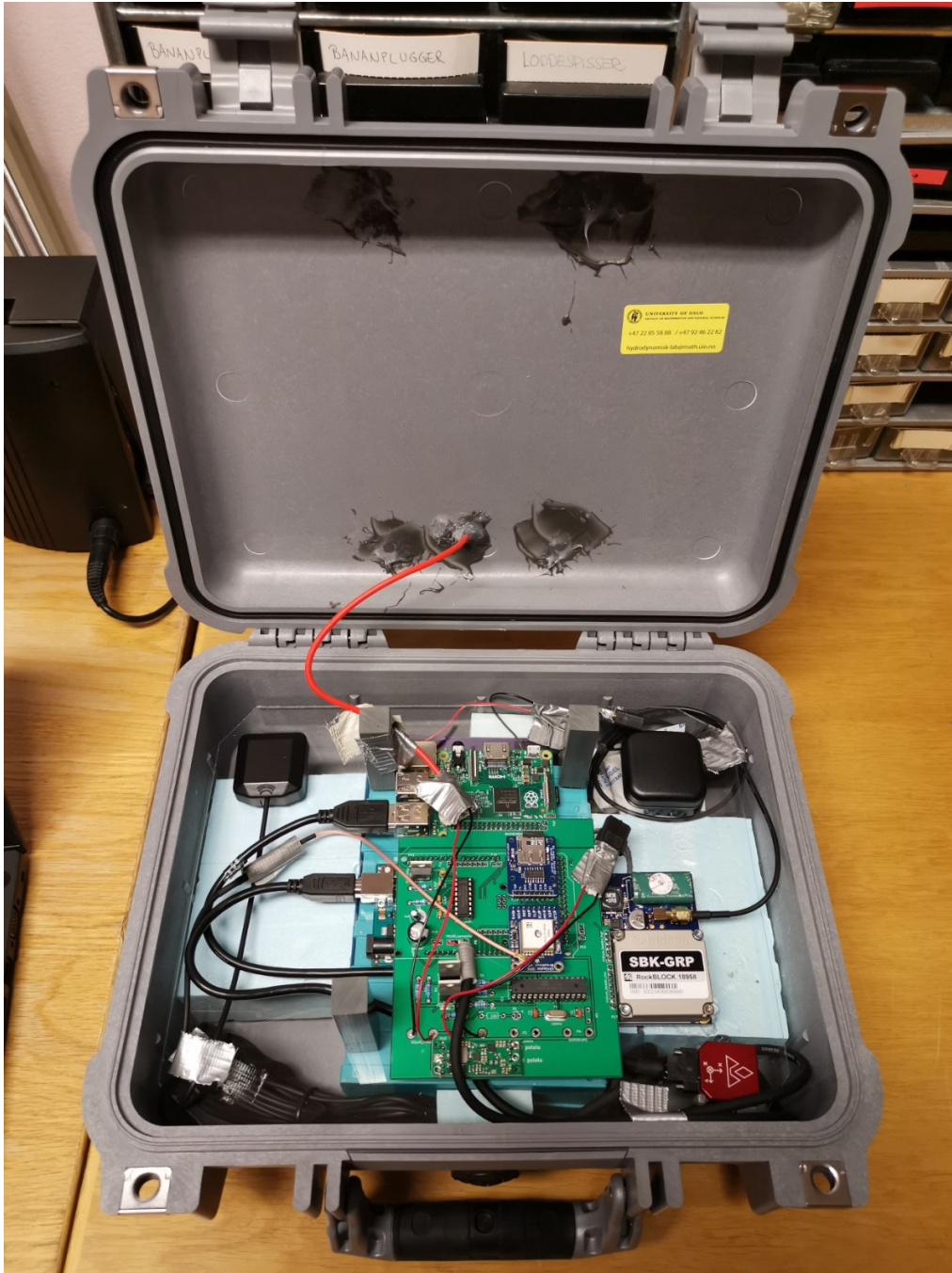
Figure 2: The instrument seen inside. The different components are clearly visible: IMU (red component at the lower right), GPS antenna (upper left), Iridium antenna (upper right), main PCB on top of an Arduino Mega including SD card reader, GPS module, and small electronics, Iridium model (right), RaspberryPi microcontroller (top), USB cable linking Raspberry Pi and Arduino Mega, single cell battery at the bottom.
