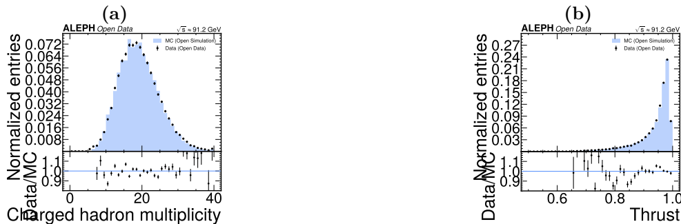
Figure 2: (a) Charged-track multiplicity, data vs MC. The distributions peak near 20 charged tracks and agree to within about 5% across the bulk, confirming that the fragmentation and tracking model entering the selection is well reproduced. A residual mean shift (data/MC scale factor 0.930) is carried as a control-observable handle (§Supporting inclusive control observables). (b) Thrust distribution, data vs MC. The event-shape variable peaks near T \approx 0.97 ; the data/MC agreement (scale factor 1.010) confirms the topology entering the hemisphere split and the polar acceptance is well modelled.
