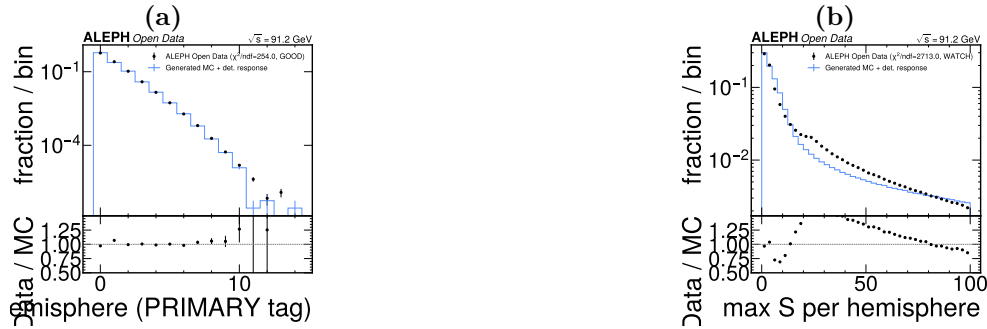
Figure 35: (a) MVA input n_{\text{hiSig}} , data vs MC (scale factor 1.022, KS 0.016). (b) MVA input \text{maxSig} , data vs MC (scale factor 0.688, WATCH).
