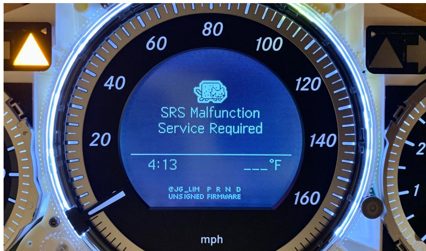
Figure 5: Successfully running unsigned firmware on the IC204
